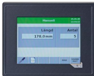
With CutLink set to Manual mode you set dimensions and the quantities. From the menu "Quick setup" you control sheet support, hold down beam and cutting sequence.
