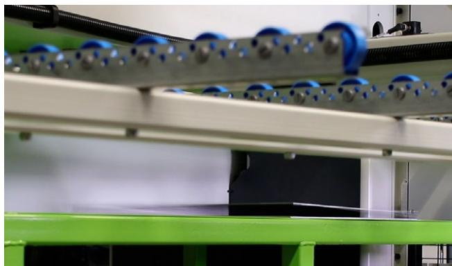
When the sheet support is pulled back, the sheets fall straight down for soft landing on the material wagon (option), with no risk of damage.
