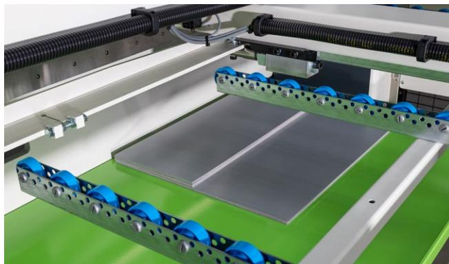
With RAPIDO SSM there is no heavy lifting. Your cut material is neatly stacked on the material wagon (option), ready for transfer to the next machine keeping panels at suitable working height.
