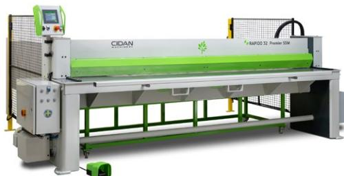
**RAPIDO SSM** (Stacking Sensitive Material) is the newly developed cut n' stack system from CIDAN machinery that speeds up your guillotine shear and never leaves you with scratches or dog-ears.
