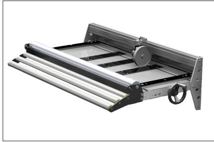
The infeed guide roller are angled to match the loop of the coil from a decoiler. This helps prevent creasing on soft materials like copper, aluminum and zinc. Another helpful feature is guiding the coil into the infeed guides. Between the slitter and shear are roller guides to ensure the material guides into the shear without curling up.
